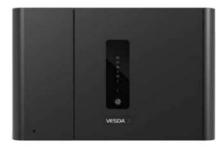
The VESDA VEP series of aspirating smoke detectors extend the reach of the VESDA platform to a wide range of applications. VEP sensitivity range is from 0.005-20%/m (0.0016-6.25%/ft) and provides up to 40 Class A holes. VEP is equipped with a powerful aspirator that provides a total of 130 m (427 ft) in the one pipe model and 560 m (1,837 ft) in the four-pipe model. VEP also provides StaX support together with Ethernet, Wi-Fi, USB and VESDAnet capabilities.
