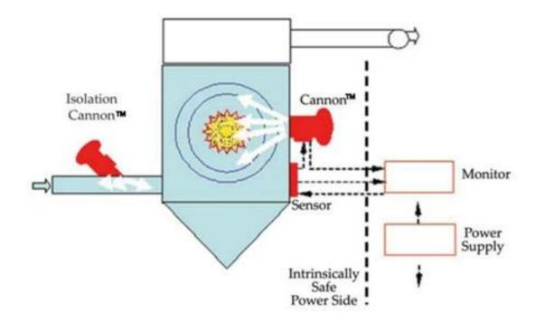
Example of a hybrid application of explosion isolation and explosion suppression: the cannon modules are employed to suppress the explosion in this dust collector and to isolate the inlet dueling providing an extinguishing barrier to burning material ns it travels through the dueling.
