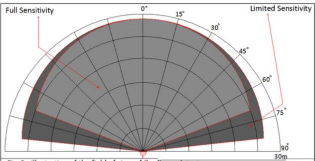
Fig. 3. Illustration of the field of view of the flame detector.
