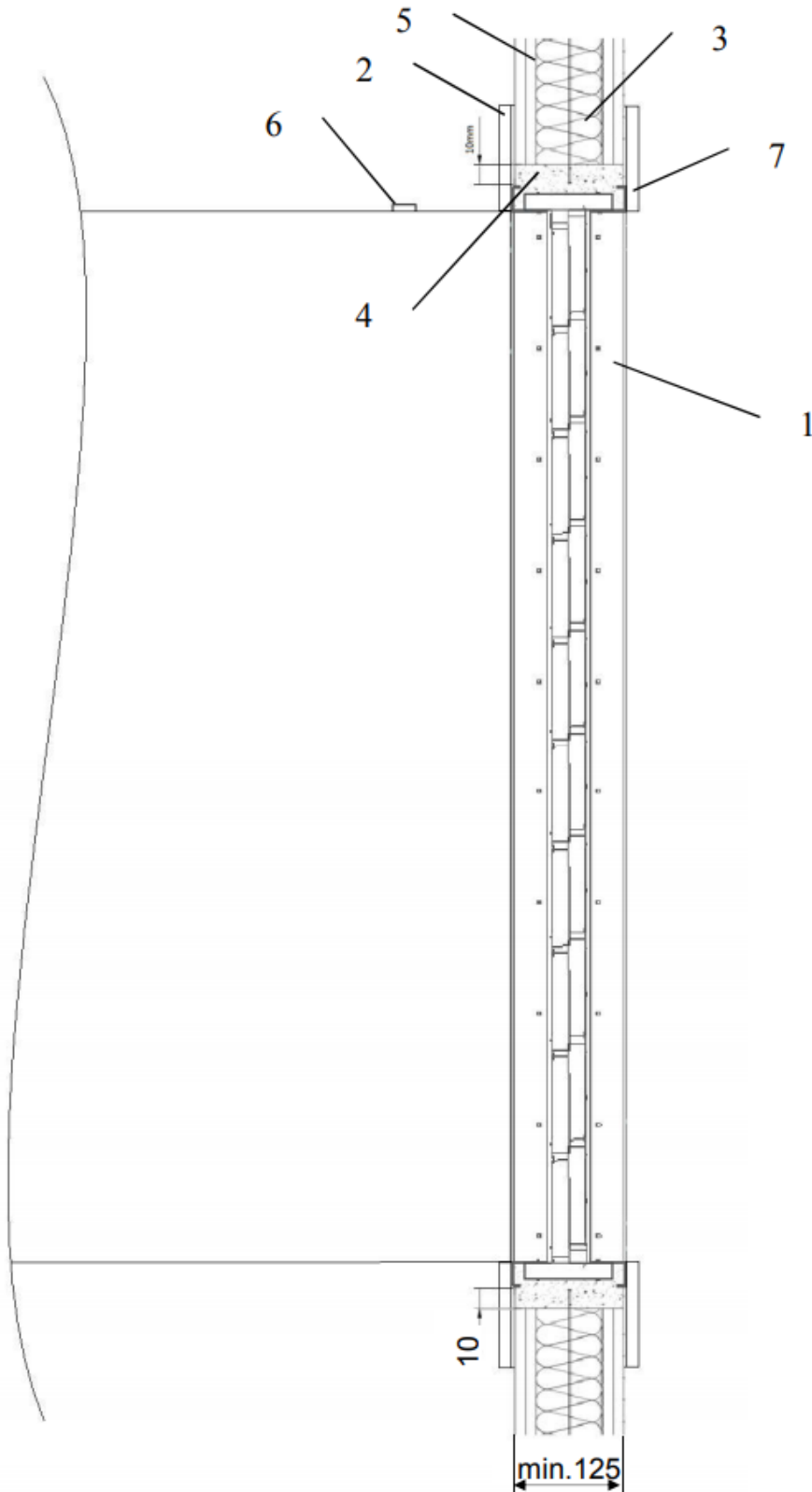
6.3.2 Fig. Installation example of the WIP PRO fire damper in a drywall structure with a minimum fire resistance rating of EI120. Installation gap: 10 mm.
